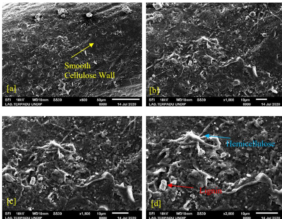
**Figure 5.** The surface morphology of specimen C2P2S: [a] MF ( $\times 500$ ); [b] MF ( $\times 1000$ ); [c] MF ( $\times 1500$ ); [d] MF ( $\times 2000$ ).
