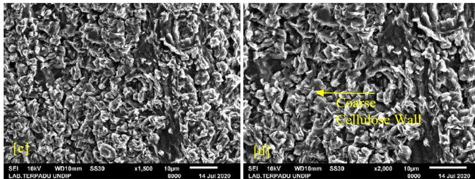
**Figure 6.** The surface morphology of specimen C6P2S: [a] MF ( $\times 500$ ); [b] MF ( $\times 1000$ ); [c] MF ( $\times 1500$ ); [d] MF ( $\times 2000$ ).
