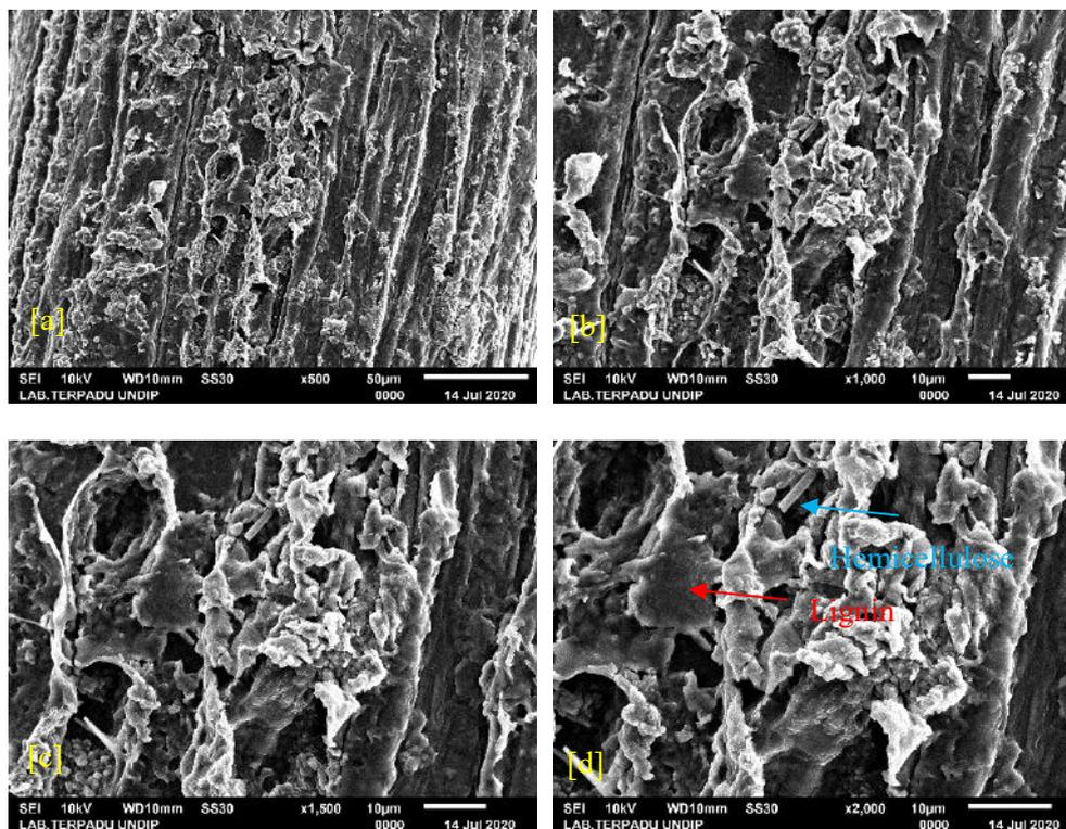
**Figure 7.** The surface morphology of specimen C0P0N: [a] MF ( $\times 500$ ); [b] MF ( $\times 1000$ ); [c] MF ( $\times 1500$ ); [d] MF ( $\times 2000$ ).
