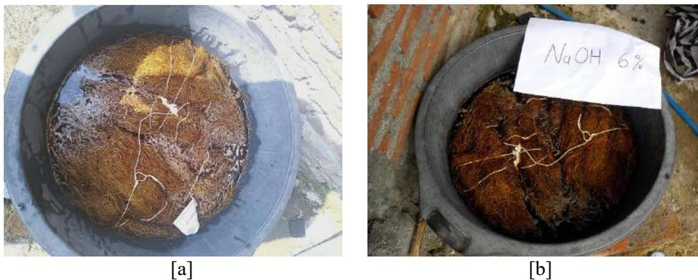
**Figure 2.** The alkali treatment of the coir fibre: [a] 2 wt% NaOH; [b] 6 wt% NaOH.
