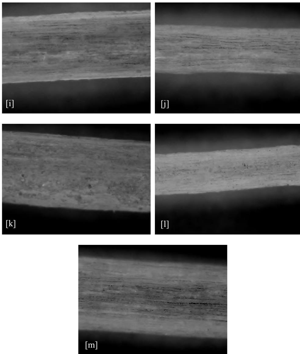
**Figure 4.** The surface morphology of the coir fibre with magnification factor 40 times: [a] C2P1O; [b] C2P1A; [c] C2P1S; [d] C2P2O; [e] C2P2A; [f] C2P2S; [g] C6P1O; [h] C6P1A; [i] C6P1S; [j] C6P2O; [k] C6P2A; [l] C6P2S; [m] C0P0N.
