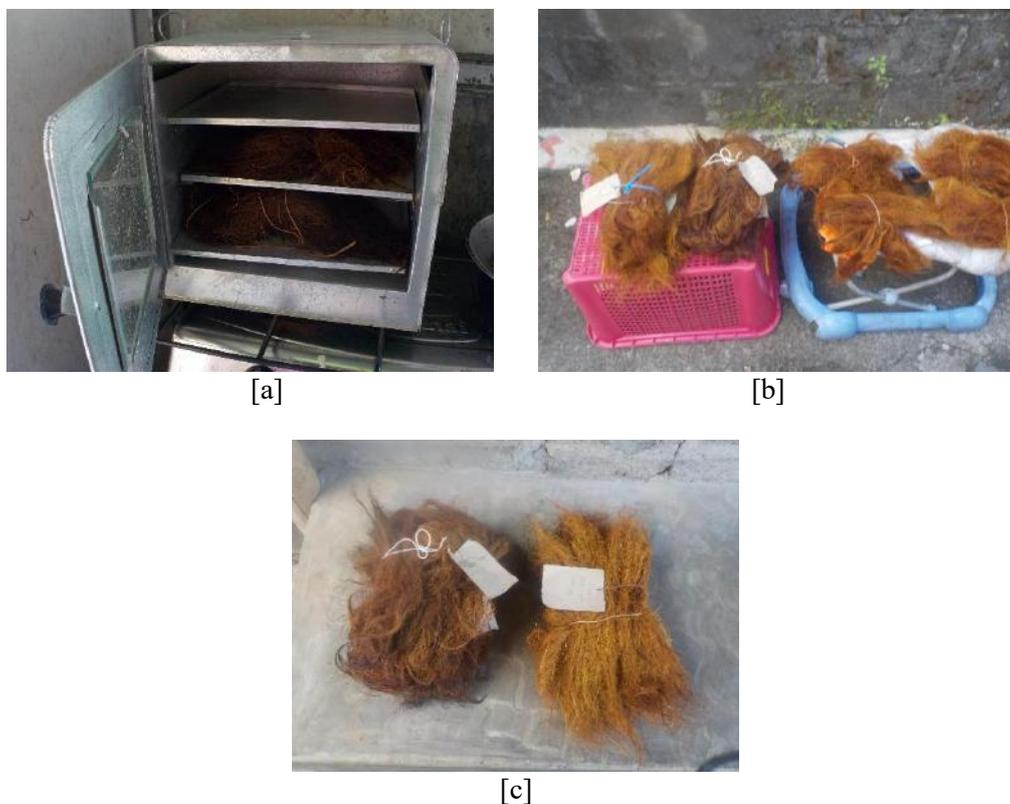
**Figure 3.** The drying method of the coir fibre: [a] oven drying; [b] air drying; [c] sun drying.
